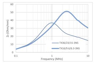
Calculating the normalized impedance Zo for both, the TX16 exhibits a wider and higher Zo due to lower eddy current losses.
