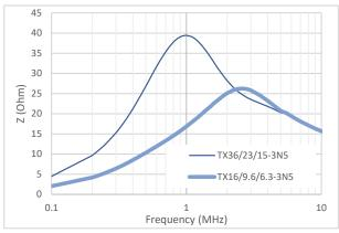
When comparing the impedance of the TX16 and TX36, the TX36 shows higher impedance mainly in the low frequency region due to its larger Ae. The TX16 performs almost the same at high frequency even though it is much smaller due to the shift in peak impedance at low frequency.
