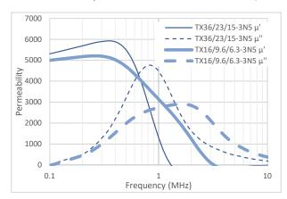
Starting from the same level of permeability, the TX16 shows wider frequency stability which reflects mainly in  $\mu$ ". This  $\mu$ " is responsible for the resistive component of the core's impedance.
