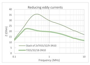
Due to the limited electrical resistivity of MnZn ferrites, the frequency bandwidth of their impedance is linked to the cross section of the core.
