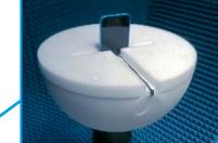
Half sphere support interface (Ø 300 mm) Includes dedicated notch to position the DUT (tablet/phone type) in vertical/horizontal position.
